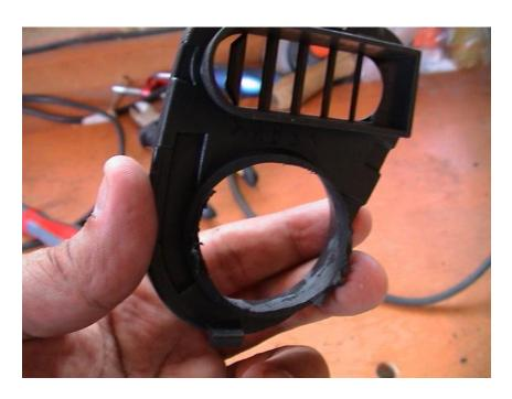
Not too much modification to do on the 0.75" tweeter then. The 1" tweeter needs a hole from nearly the edge of the housing to the air vent, and is very tricky to get it right.
