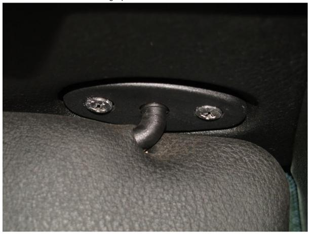
Remove the two screws that locate the front of the headlining
