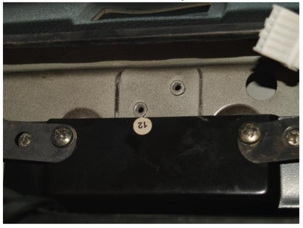
you don't need to remove the two which locate the black plate above it. Now the front of the headlining can be gently bent downward. I \*think\* that if you wish you can remove the trim around the sunroof opening to improve access but I haven't found it necessary.
