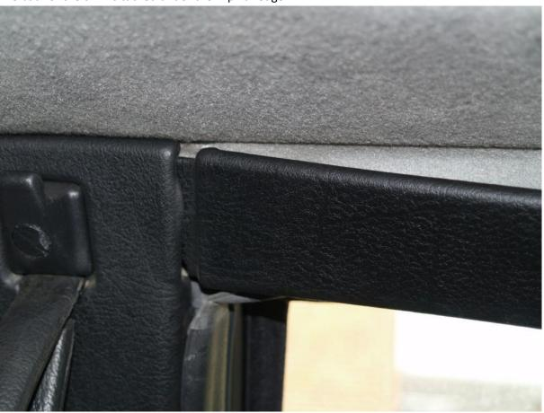
Remove the sunshades and retaining clips from both sides.
