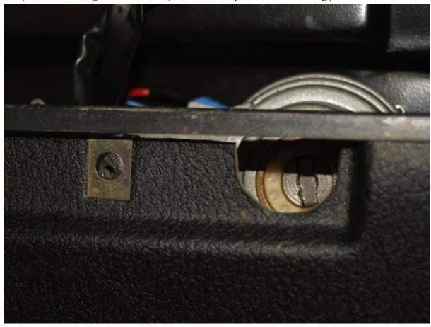
but this is not necessary to access the large screw-head visible through the circular cut-out. It's not apparent that this is a screw-socket since there's a spring-located internal cover, but poking it with a large screwdriver will yield dividends.
