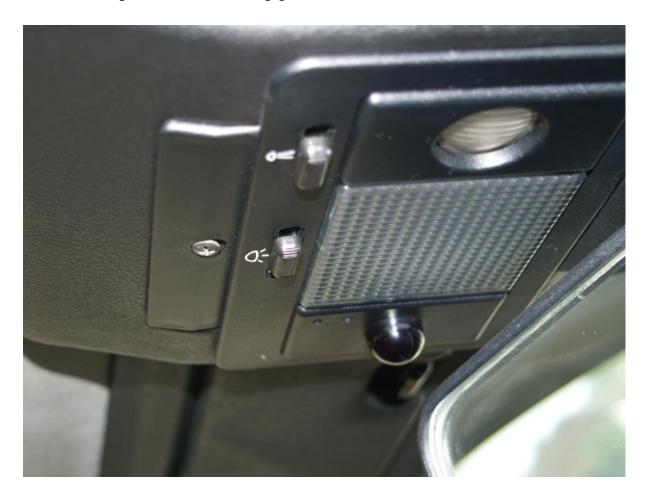
Here's the light unit; the small plastic plate at the back can be removed along with the single screw.
