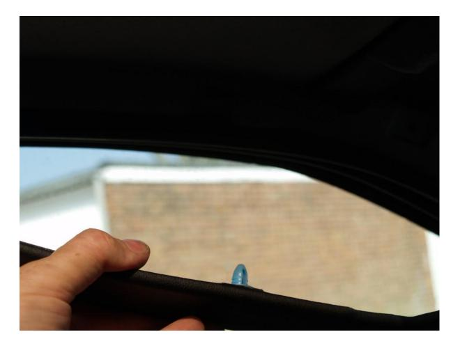
The back of the trim is tucked under the A-pillar edge.
