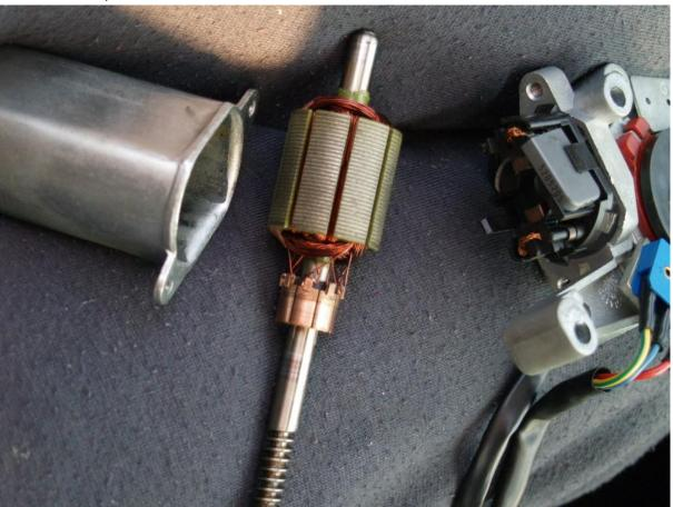
the casing (removed by undoing two screws), the rotor, and the gearbox, brushes, and switches. Clean the commutator and make sure the separations between the copper segments aren't full of carbon from the brushes. You'll want to ensure that the axle is greased where it goes into its bearing at the back of the housing, the front bearing, and the worm drive.
