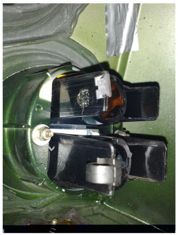
Twist the two bulb units out and then the light assembly can be extracted out of the surround
