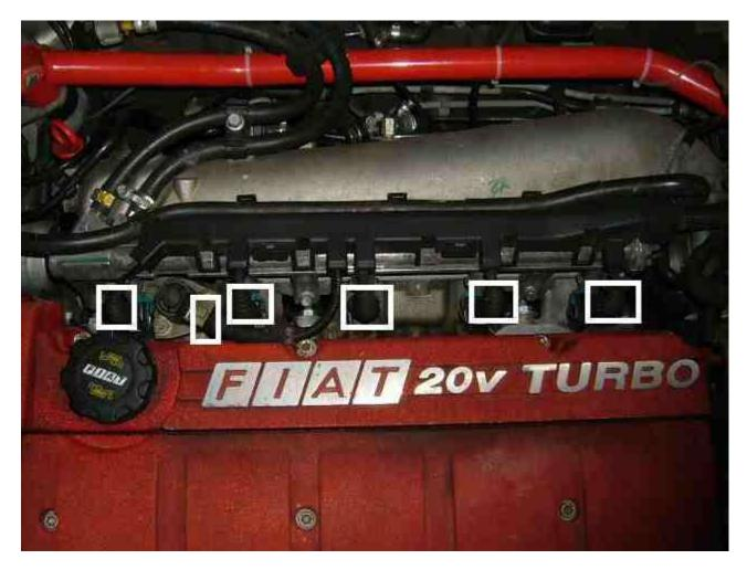
Then undo the hose from the coolant header tank and the fuel hose clip on the back of the intake manifold, as shown:
