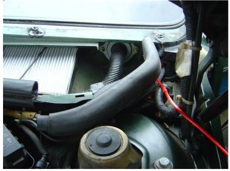
Then you will need to unbolt the top three bolts in the wing under the sponge bit and carefully prise the wing away. You will see the wire which can then be passed into the Cabin through the hole shown. You should also ensure the wire is sheathed or a proper rubber grommet is fitted around this hole to prevent chaffing.
