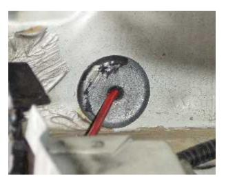
5. Working inside the car now. Pull off the door seal and lift the carpets away, underneath is another handy grommet. You will of course have to feed the cable down with a wire and string.
