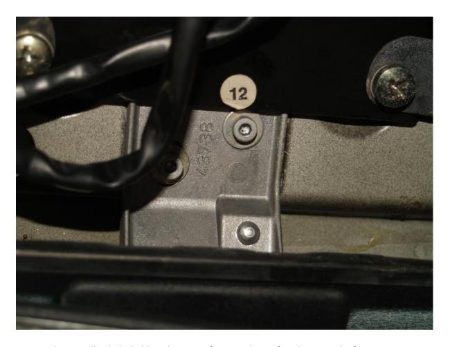
Remove the two Allen bolts holding the mirror frame to the roof, and remove the frame.
