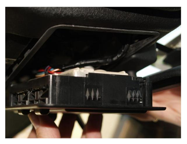
Slide the light unit to the left and allow the right hand side to drop out of the fixture; disconnect the wires and remove.
