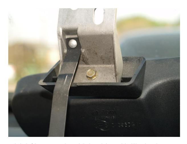
On the back of the mirror is a single 7mm bolt; this works loose and should be tightened.
