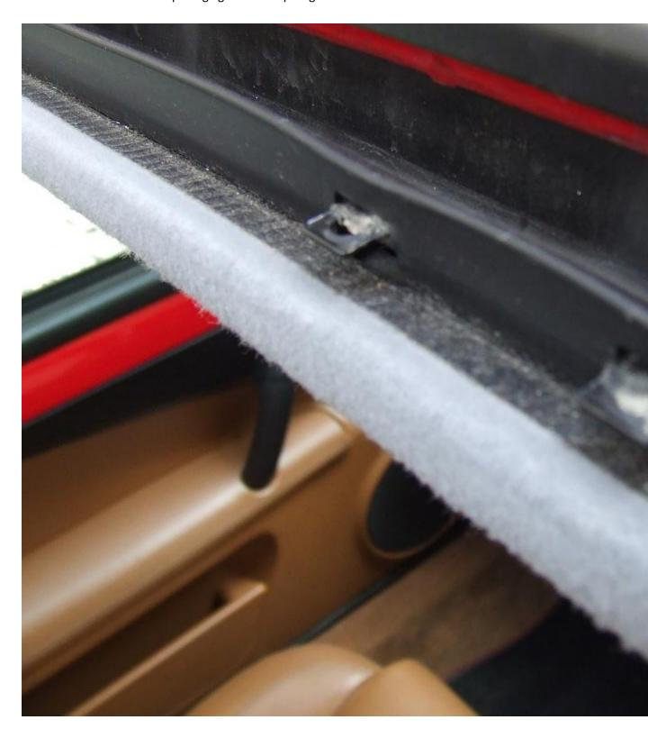
And against this metal strip the vent screen slides under when open.
