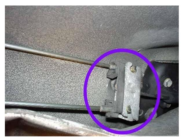
Now release the ends of the cables from the tie bar. This is in the middle of the car underneath and is easily accessible. Just remove the plastic clip and turn the cable ends out of the slots.
