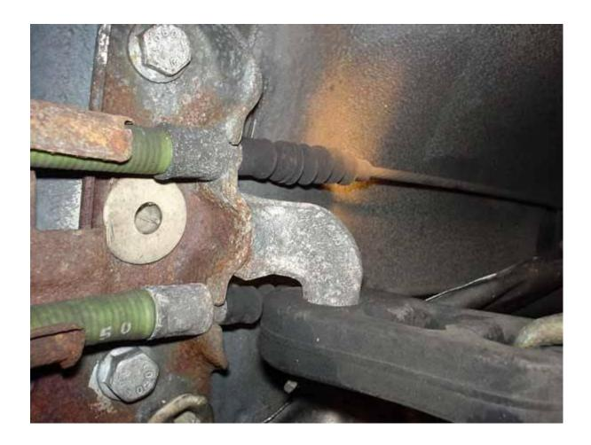
Working towards the rear of the car, simply pull the cable assembly rearwards from these supports.
