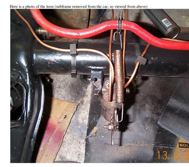
The idea is that under hard braking as the nose of the car dips, and the rear rises, the valve reduces pressure to the rear callipers to prevent the brakes from locking. So if the valve has seized in this position foot brake efficiency at the MOT will be poor. It is worth checking the condition of the rubber boot occasionally and giving the area behind the boot a good spray of copper grease every year or so..
