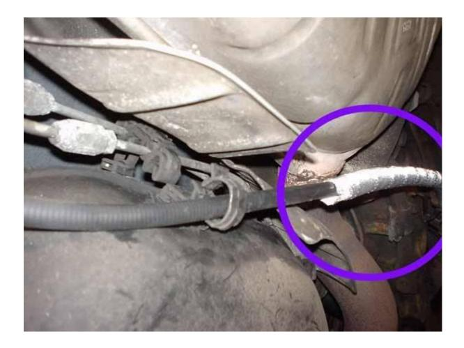
On the exhaust side you'll find this aluminium sheath which protects the exposes section from heat damage.
