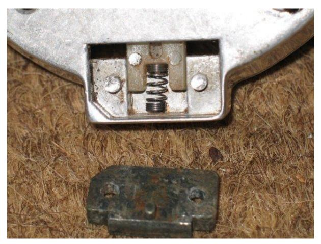
This shows the little knob on the back of the metal plate that keeps the plastic clip from being pushed out too far by the spring.
