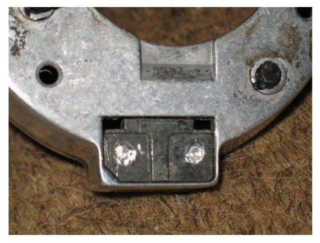
You want to drill just enough to remove the "lip" of metal that keeps the plate in place.
