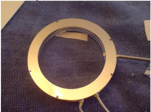
3. Cut slots so cable can come straight back instead of down
